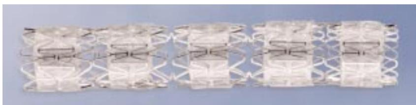
**Figure 41.1:** The Quanam QueST stent consists of individual segments each 3.8 mm long joined by inter-segment connecting links. On the QuaDDS-QP2 stent a non-biodegradable proprietary polymer is ensheathing the QueST stent loaded with the slow-release microtubular inhibitor 7-hexanoyltaxol ('taxen').
